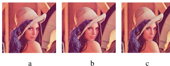
Figure 4. Simulation Results of Transform, Quantization and CAVLC Processors for H.264 Video Encoder a Original Lena image (512x512 pixels) b Reconstructed Lena Image using Matlab, PSNR: 37.1 dB c Reconstructed Lena Image using Verilog, PSNR: 37.3 dB
