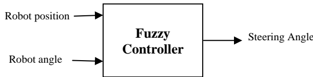
Figure 5. Structure of the proposed control system.
