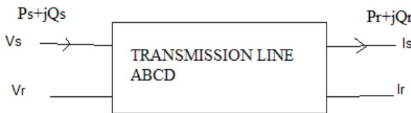
Figure 1. Two port four terminal model of a transmission line.
